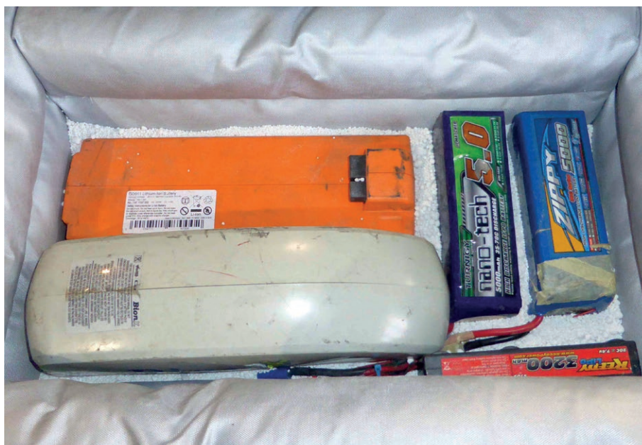
Figure 4: Fireproof box with a refractory lining material (PyroBubbles®) provided by Inobat for visibly damaged (swollen) or overheated lithium-ion batteries
