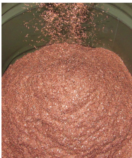
Figure 2: Copper granulate from cable recycling
